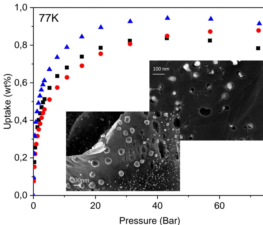
**Figure 1.** H<sub>2</sub> uptake isotherms recorded at 77K for Pd decorated samples prepared according to procedure described by H.Kumar *et al.* using microwave exfoliation and air etching: precursor r-GO prepared using microwave exfoliation (▲), Pd decorated and microwave treated r-GO (●), Pd decorated air annealed r-GO (■). Inset shows SEM images of r-GO decorated with Pd nanoparticles. Air-annealed samples show holes etched around Pd nanoparticles similarly to ref 1.
