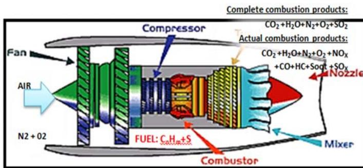
Figure 3: Turbine engine diagram with combustion products.
