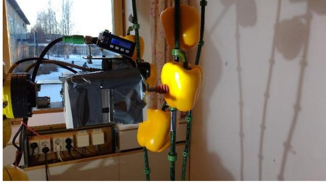
**Fig. 5.** The pose of each pepper was measured by manually moving the robotic arm in the desired approach direction to the position where the gripper touched the fruit.
