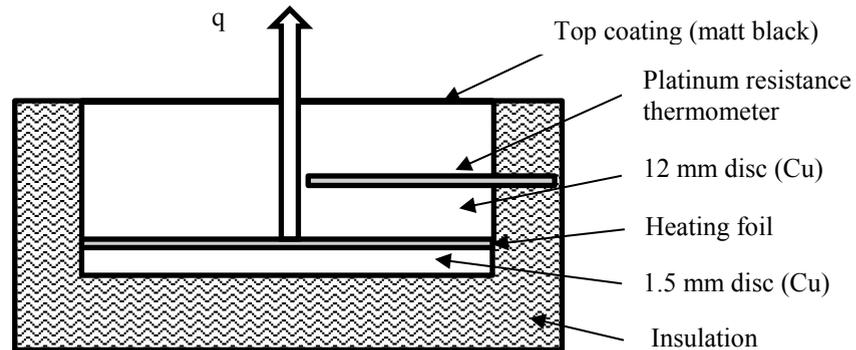
Fig. 1. Solar air thermometer (SAT) unit.
