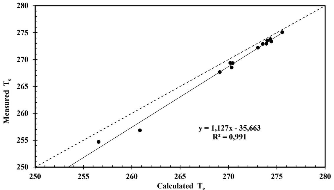
Fig. 3. Comparison of the resulting  $T_{e,calc}$  and  $T_{e,meas}$  based on the nine measurement periods.
