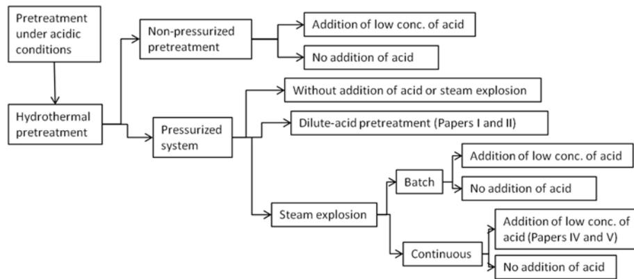
**Fig. 4** Acid-based pretreatment. The type of pretreatment used in the studies described in Papers I, II, IV, and V are indicated.
