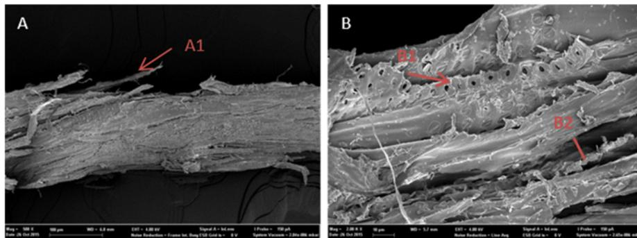
**Fig. 6** SEM images providing an overview of a piece of aspen wood (A, magnification 500  $\times$ ), and detailed surface characters (B, magnification 2000  $\times$ ). A: Aspen wood cells gathered together as a loose structure with some dispersed fibers (A1). B: Pits (B1) indicates the exposed cell lumen of a broken wood cell, and (B2) the wide gap between fibers confirming the loose structure of aspen wood.
