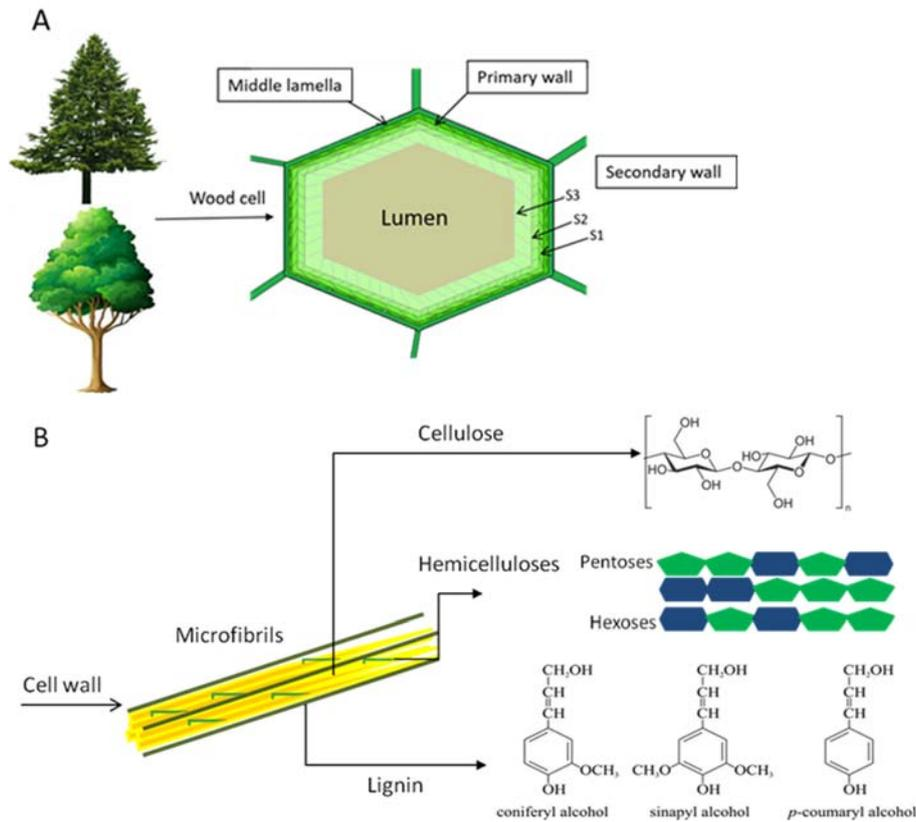
**Fig. 2** Multilayer structure of wood cell walls (A), and major constituents of wood (B).
