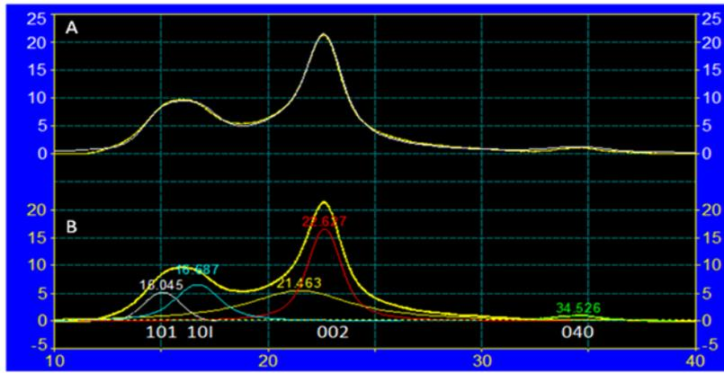
**Fig. 5** XRD analysis for measuring the crystallinity of a wood sample. A: Spectrum from the XRD analysis. B: Curve-fitting process with Gaussian function for the cellulose crystalline peaks (101: 15.045;  $10\bar{1}$ : 16.687; 002: 22.627; and 040: 34.526) and for the amorphous region (21.463).
