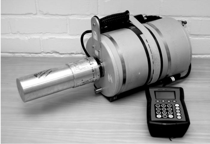
**Figure 5.** One of the HPGe detectors used (Detector 2, 57% efficiency) and the DigiDART portable MCA.
