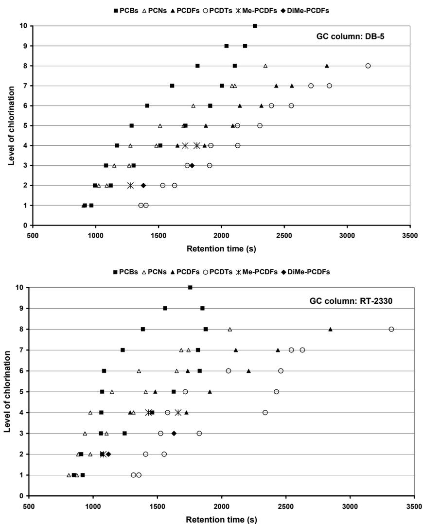
**Figure 10.** Elution windows for PCBs, PCNs, PCDFs, PCDTs, methyl-PCDFs, and dimethyl-PCDFs on a DB-5 (top) and an RT-2330 (bottom) fused-silica capillary column.
