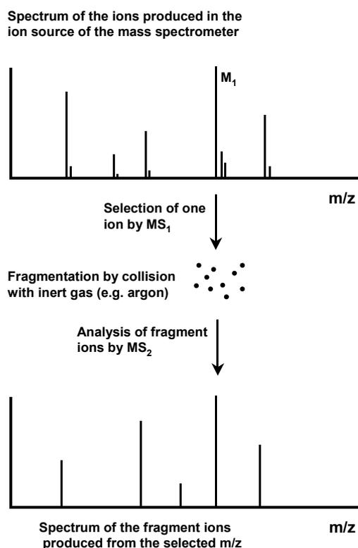
**Figure 11.** Principle of MS/MS: an ion,  $M_1$ , is selected by the first spectrometer,  $MS_1$ , fragmented through collision and the fragments are analysed by the second spectrometer,  $MS_2$ .
