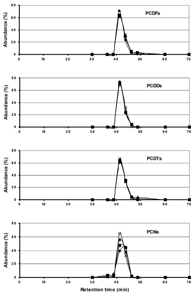
**Figure 9.** Elution profiles of PCDFs, PCDDs, PCDTs, and PCNs on the 100-mg HPLC PX-21 carbon column. Legends for degree of chlorination: ×, hepta; ▲, hexa; ■, penta; ◆, tetra.
