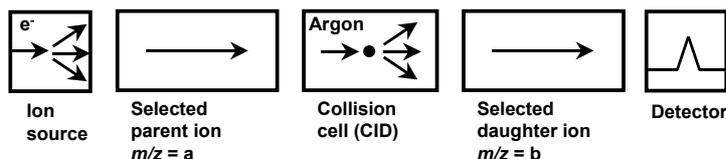
**Figure 12.** Processes in selected reaction monitoring scan mode.
