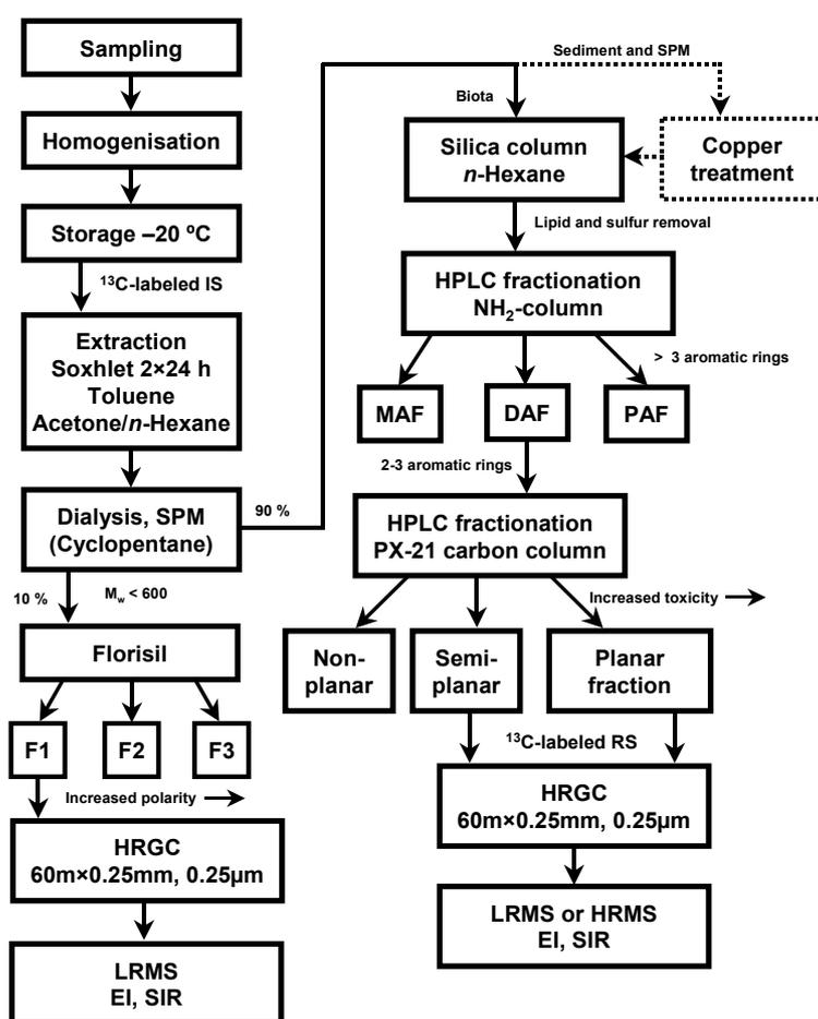
**Figure 8.** Analytical flow diagram, showing principal cleanup and analysis steps for PCBs, PAHs, planar dioxin-like pollutants (e.g. mono-*ortho* PCBs, non-*ortho* PCBs, PCNs, PCDTs, and R-PCDFs), and PCDD/Fs.
