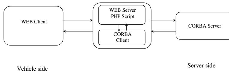
Figure 6: Simulating networked driver mental state surveillance system. The left side is the web client, which act like the vehicle side, the right side is the server side.
