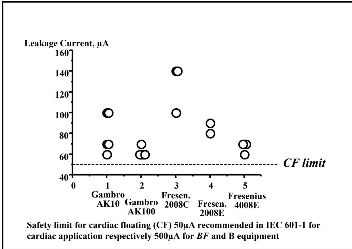
Figure 9: Plots for each measurement of leakage current for different devices- patient leakage current - single fault condition.
