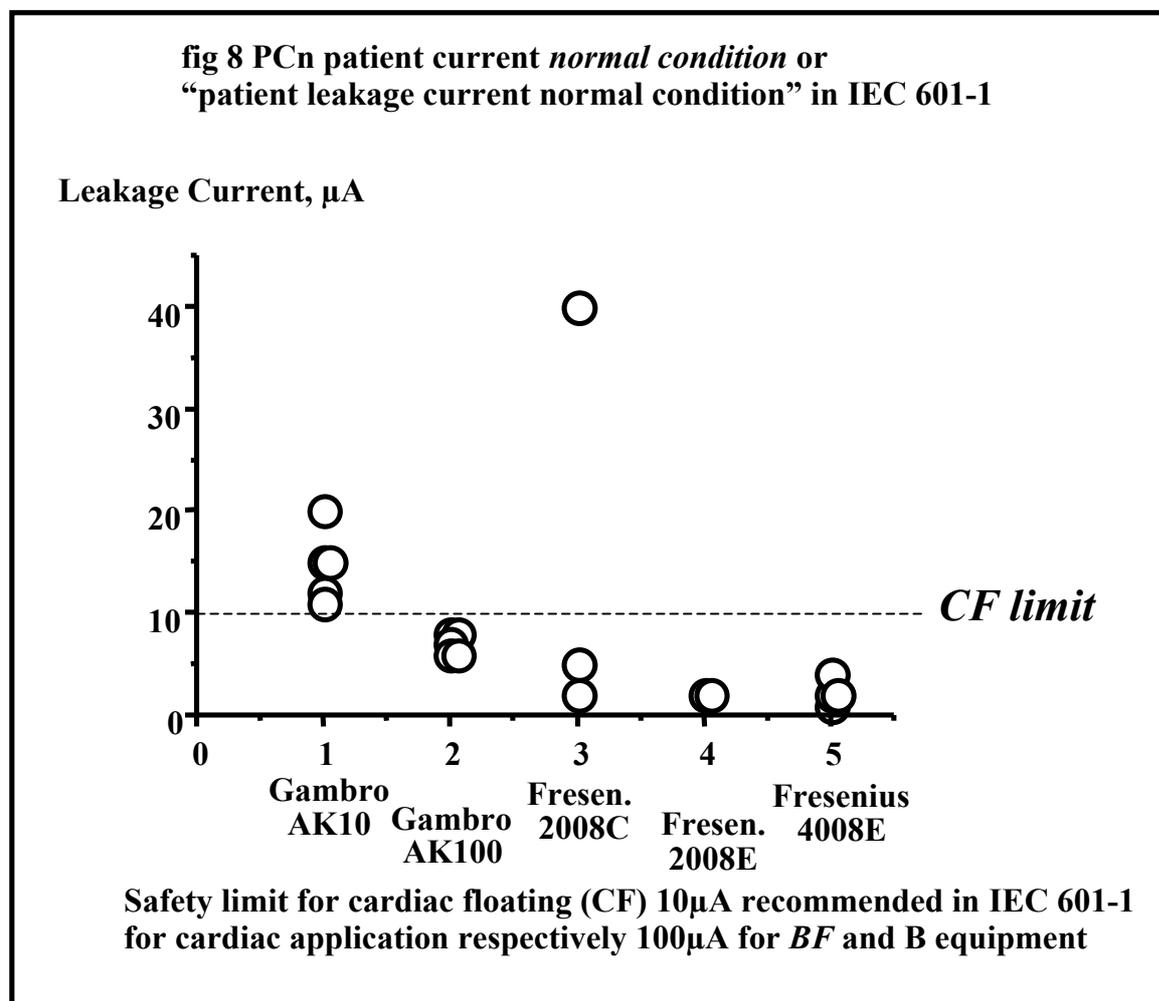
Figure 8: Plots for each measurement of leakage current for different devices-normal condition. (The dot at  $40\mu\text{A}$  at 2008C is a high value due to a failure in a capacitor in a conductive level detector in the fluid system. After service the leakage current in normal condition was  $3\mu\text{A}$  the following two years. The value after repair,  $3\mu\text{A}$ , was used in the paper I statistic.)
