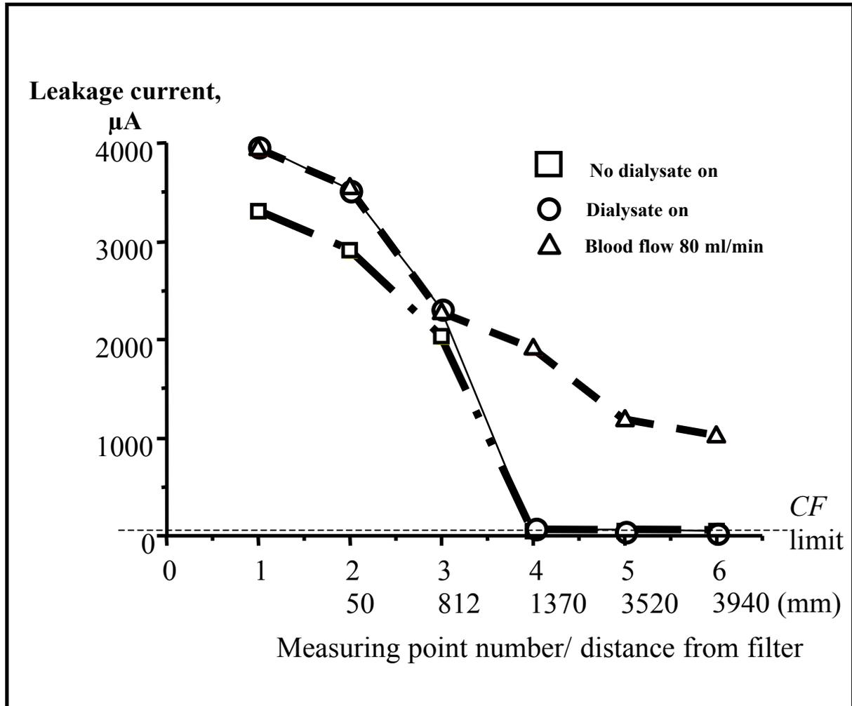
**Figure 14. Leakage current using blood in blood lines and testing *mains on applied part***
