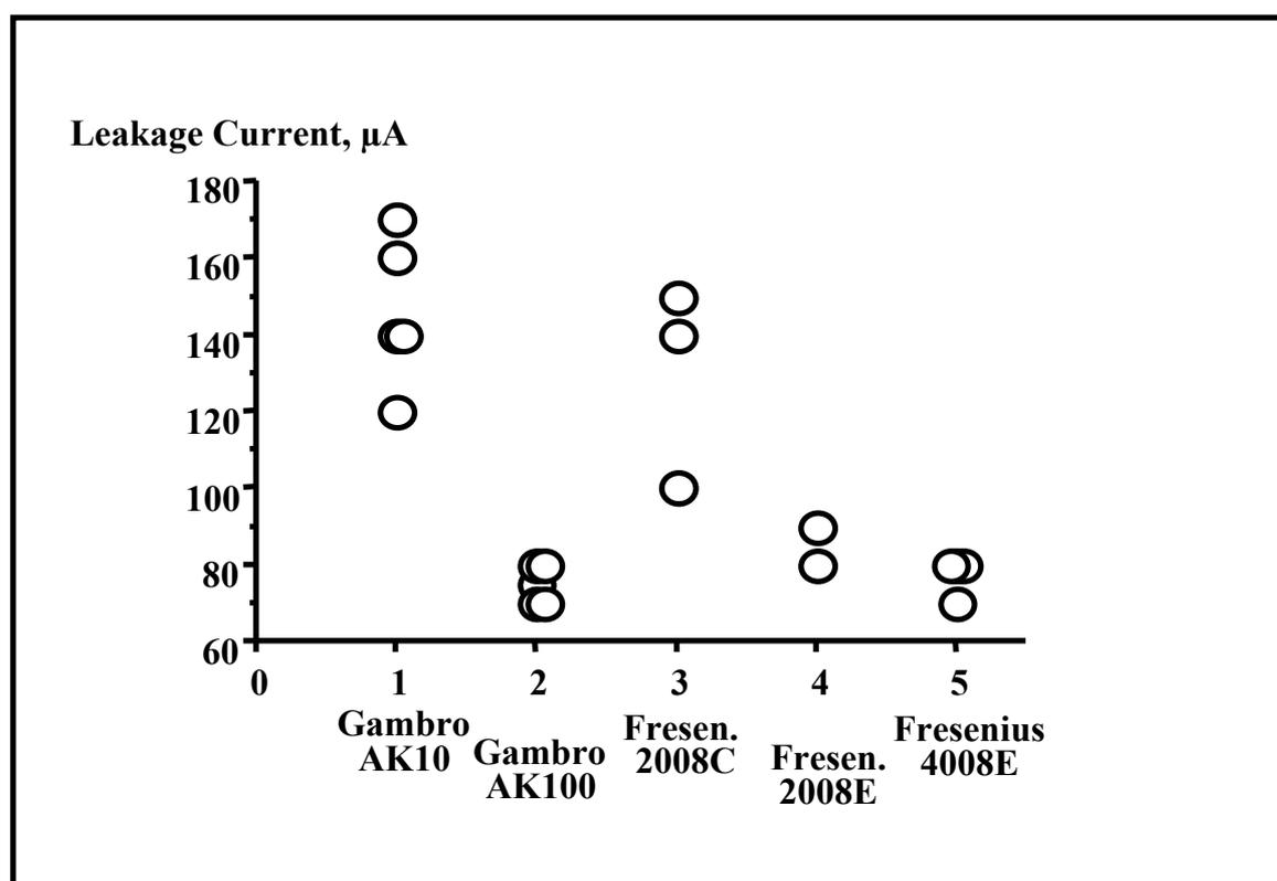
**Figure 8. PCn patient current, normal condition or patient leakage current normal condition in IEC 601-1**
