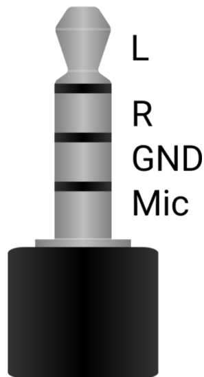
Figure 5 – Tip, Ring, Ring, Sleeve plug (CTIA) Wikimedia commons.
