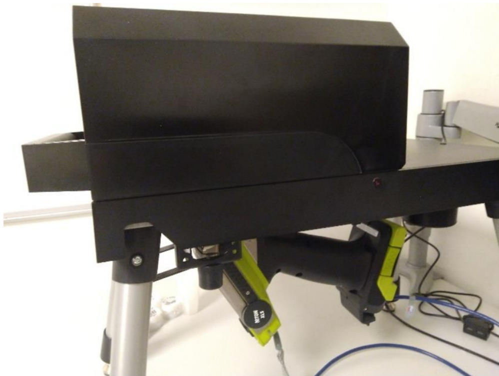
Figur 12 The portable Energy Dispersive Thermo Scientific Niton XL 5 was used for XRF measurements, attached to a test stand.
