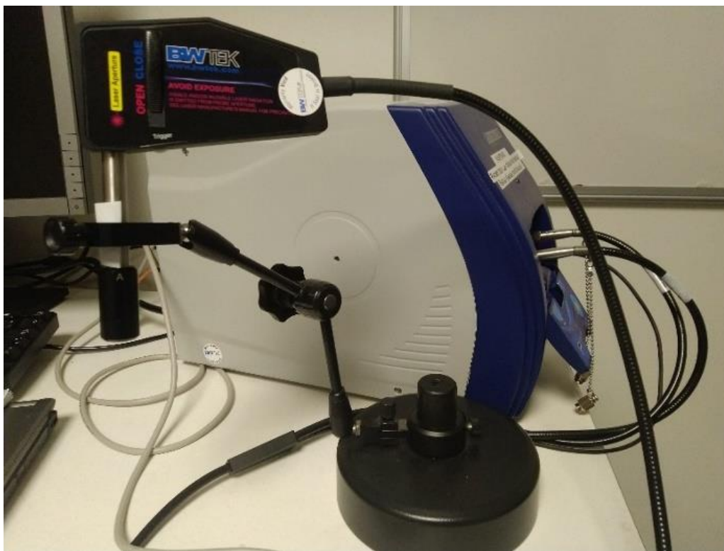
Figure 11 The i-Raman EX was used for Raman measurements, with a 1064 nm excitation laser.
