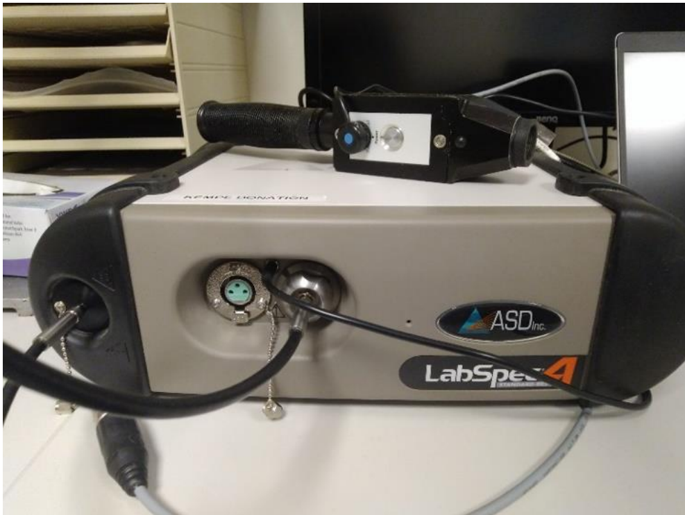
Figure 10 The ASD LabSpec 4 was used for for NIR measurements, with a contact probe for sampling.
