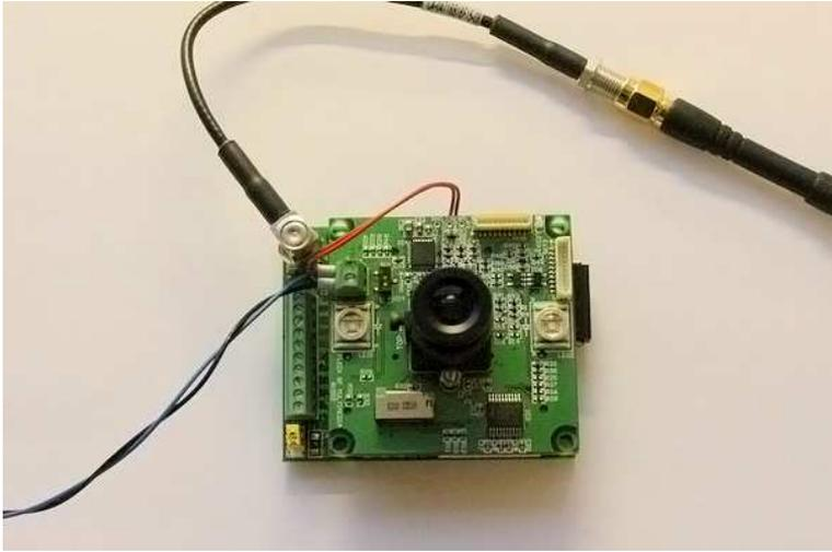
**Fig. 5.2:** Illustration of camera stack formed by a Fleck<sup>TM</sup>-3 sensor node, AD Blackfin board and CMOS camera.
