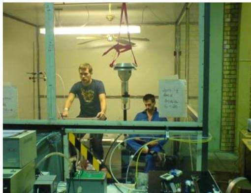
program with acceleration and breaking is called the European Transient Cycle (ETC), where the urban part of the program was used (fig 3). The monitoring and the technique to feed the chamber with the exhaust were the same as in study 1. In study 2 and 4 the mass concentration was
