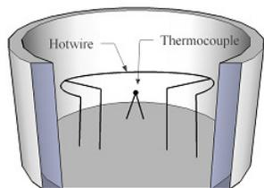
**Fig. S1.** Teflon sample cell with the hot-wire probe and thermocouple for high-pressure in-situ measurements of thermal conductivity and heat capacity per unit volume.
