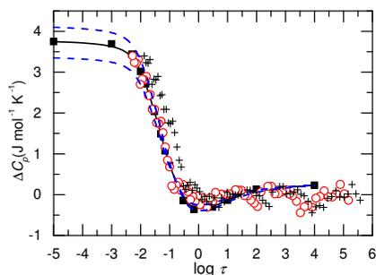
Fig. S5. Heat capacity change as a function of the logarithm of the relaxation time (in s): (+) results of measurements plotted against the dielectric relaxation time and (O) the same data but shifted  $\Delta \log \tau = -0.4$  to coincide with the calculated values (■) (see text). The dashed lines provide an error estimate.
