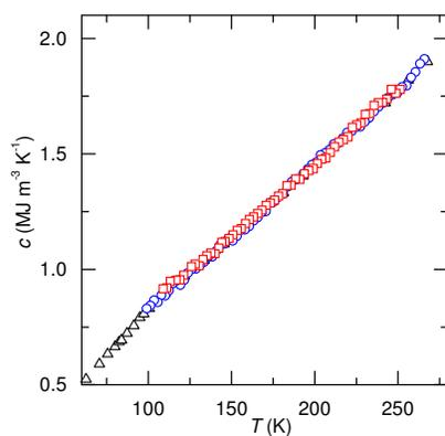
**Fig. S2.** Heat capacity per unit volume of hexagonal ice at  $\sim 0.05$  GPa plotted against the temperature. (□) and (○) are the data obtained in two experiments by using 0.3 mm diameter hot-wires. (△) are the values determined from  $C_p$  data (4) and density (5). At  $T > 120$  K, the values agree to within 2%. At  $T < 110$  K, interference with the reflection of the heat wave from the cell wall added to the uncertainty in the measurements.
