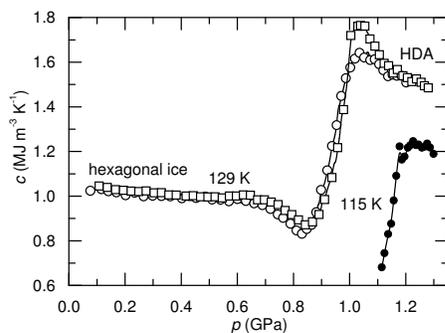
**Fig. S6.** Heat capacity per unit volume plotted against temperature pressure at 129 K and 115 K. The 115 K data, which have not been previously published, were obtained using a 0.1 mm hot-wire probe in a study in 2004 [11]. The 0.1 mm probe gives erroneous results for ice Ih due to the high thermal diffusivity, and the low-pressure data have therefore been removed.
