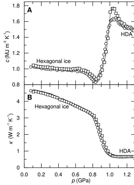
**Fig. 1.** Thermal properties prior, during and after pressure collapse of hexagonal ice, ice Ih. (A) Heat capacity per unit volume, and (B) Thermal conductivity on isothermal pressurization at  $(129 \pm 1)$  K. The squares and circles show results for two different runs, which agree to within 2% outside the collapse range.
