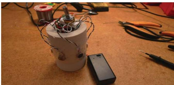
Figure 2. A grip with 7 vibrators, with manual control.
