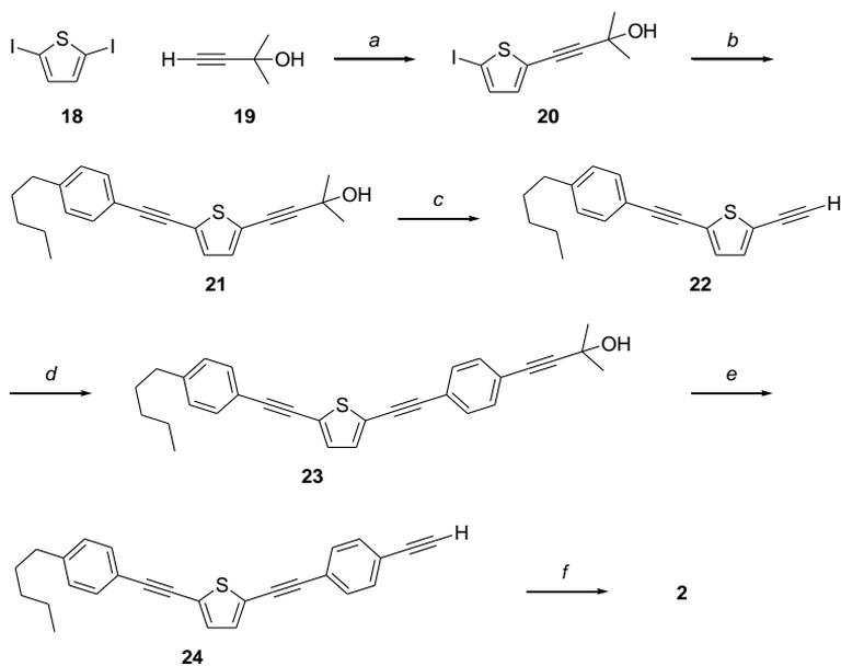
**Scheme 3.** Synthesis of compound **2**. *a*) Pd(PPh<sub>3</sub>)<sub>2</sub>Cl<sub>2</sub>, CuI, PPh<sub>3</sub>, THF/Et<sub>3</sub>N (68%); *b*) Conditions as *a* (86%); *c*) NaH, toluene (29%); *d*) Conditions as *a* (70%); *e*) KOH, toluene (66%); *f*) *trans*-Pt(PBu<sub>3</sub>)<sub>2</sub>Cl<sub>2</sub>, CuI, Et<sub>3</sub>N/THF (72%).
