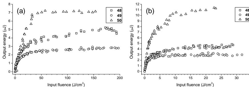
**Figure 16.** OPL of compounds **48-50** (30 mM in THF) at (a) 532 nm and (b) 600 nm.
