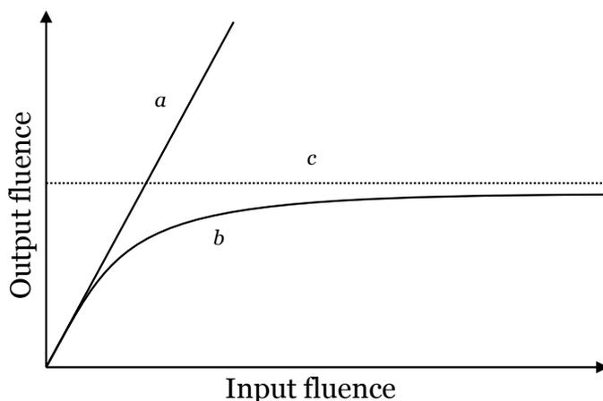
**Figure 2.** Schematic energy diagram showing the behaviour of an OPL material. *a*) Linearly absorbing material. *b*) OPL material. *c*) Clamping level.
