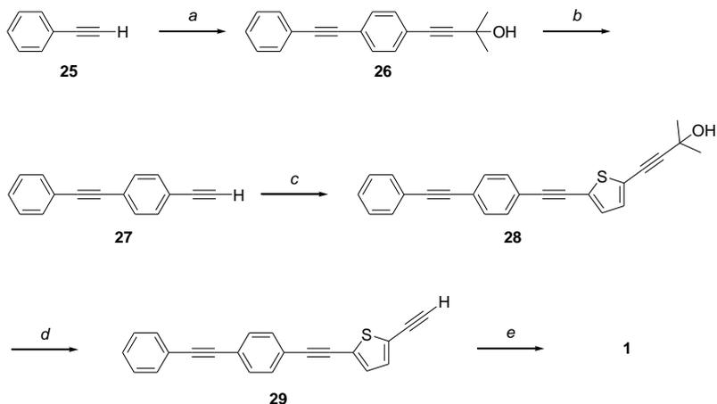
**Scheme 4.** Synthesis of compound **1**. a) **7**, Pd(PPh<sub>3</sub>)<sub>2</sub>Cl<sub>2</sub>, CuI, PPh<sub>3</sub>, THF/Et<sub>3</sub>N; b) KOH, toluene (63% over two steps); c) **20**, Pd(PPh<sub>3</sub>)<sub>2</sub>Cl<sub>2</sub>, CuI, PPh<sub>3</sub>, THF/Et<sub>3</sub>N (60%), d) Conditions as b (78%); e) *trans*-Pt(PBu<sub>3</sub>)<sub>2</sub>Cl<sub>2</sub>, CuI, Et<sub>3</sub>N/THF (86%).
