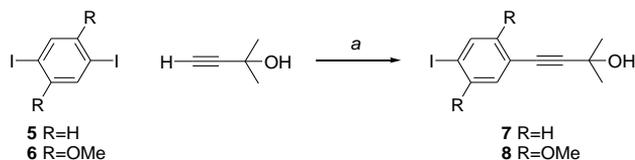
**Scheme 1.** Synthesis of building blocks **7** and **8**. a) Pd(PPh<sub>3</sub>)<sub>2</sub>Cl<sub>2</sub>, CuI, PPh<sub>3</sub>, DMF/Et<sub>3</sub>N (45% and 47% respectively).
