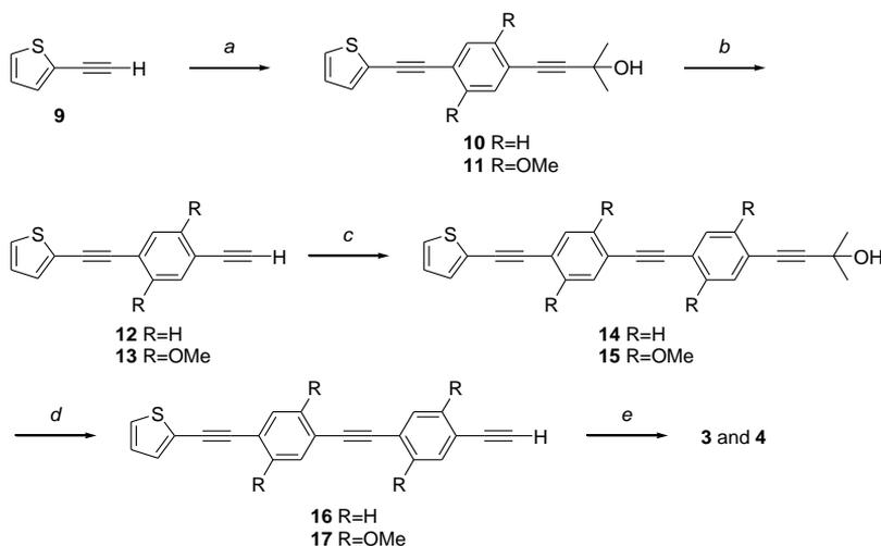
**Scheme 2.** Synthesis of **3** and **4**. a) **7** or **8**, Pd(PPh<sub>3</sub>)<sub>2</sub>Cl<sub>2</sub>, CuI, PPh<sub>3</sub>, THF/Et<sub>3</sub>N (89% for both compounds); b) KOH, toluene (89%; 84%); c) Conditions as a (88%; 64%); d) Conditions as b (98%; 87%); e) *trans*-Pt(PBu<sub>3</sub>)<sub>2</sub>Cl<sub>2</sub>, CuI, Et<sub>3</sub>N/THF (quant.; 60%).
