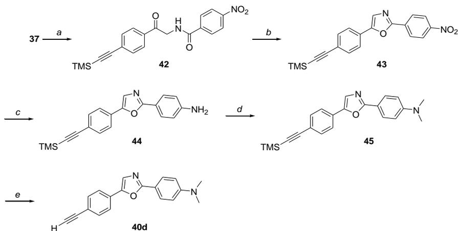
**Scheme 7.** Synthesis of compound **40d**. a) 4-nitrobenzoyl chloride, Et<sub>3</sub>N, CH<sub>2</sub>Cl<sub>2</sub> (62%); b) POCl<sub>3</sub>, DMF (47%); c) Zn, AcOH (86%); d) MeI, DMF (85%); e) K<sub>2</sub>CO<sub>3</sub>, MeOH (79%).
