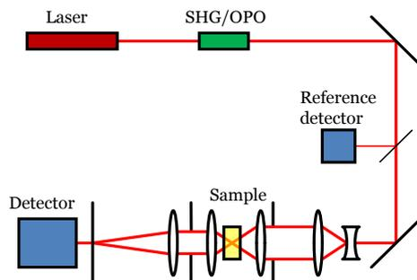
**Figure 3.** Schematic OPL measurement setup.
