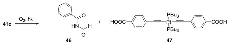
**Scheme 8.** Degradation of compound **41c** in air and light.
