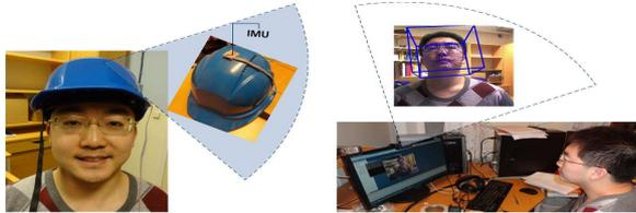
Figure 3: (a) IMU Based head pose estimation (b) CLM plus Geometric Based Sol.
