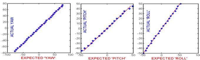
Figure 4: Expected Vs Actual angles for (a) Yaw (b) Pitch (c) Roll
