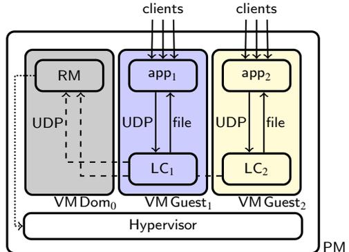
Figure 2: Architecture of a single Physical Machine (PM).
