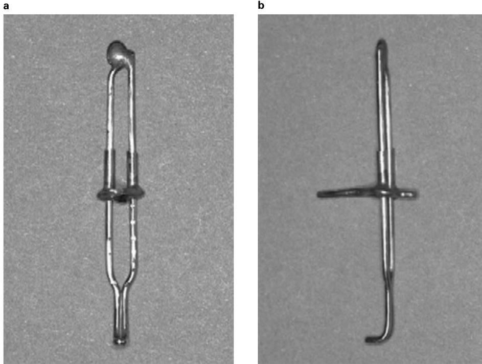
**Figure 2** The specially constructed caliper for increasing the distance from the alveolar crest to the mental foramen shown from the front (left) and side (right).
