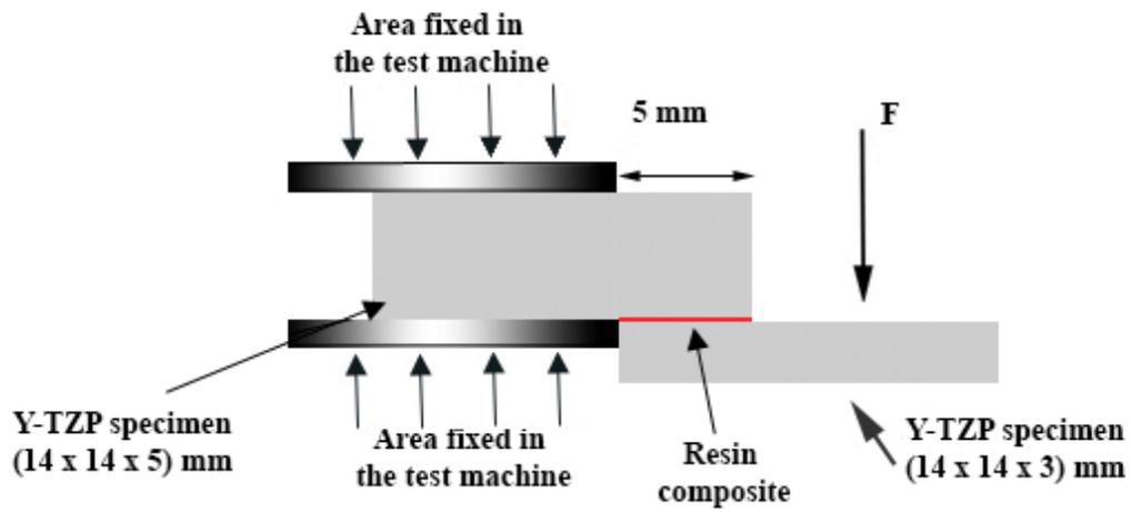
Fig. 2. Schematic drawing of the specimens placed in the testing machine.
