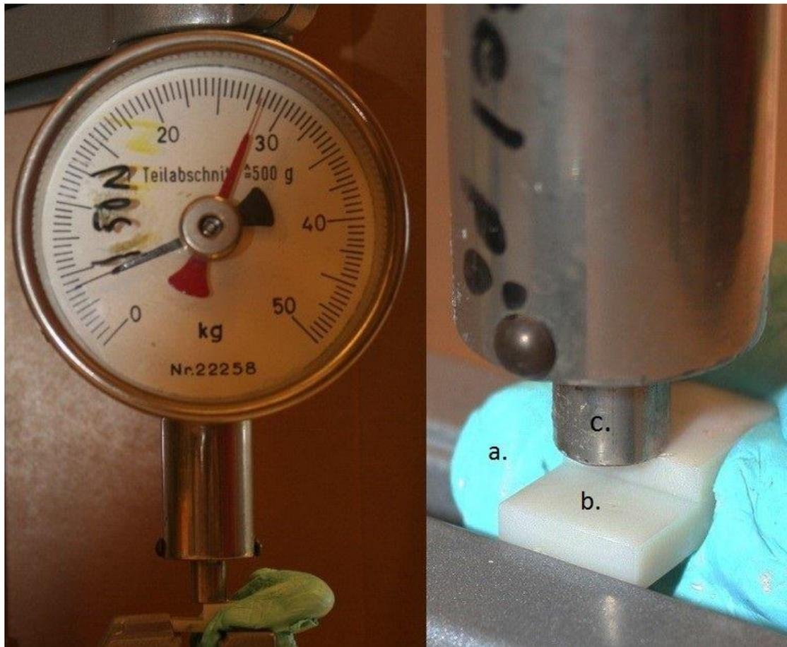
Fig. 1. The specimens placed in a mold of a vinyl polysiloxane impression material (a.) during the cementation procedure. The cemented pair of zirconia specimens (b.) being loaded by a plunger (c.).
