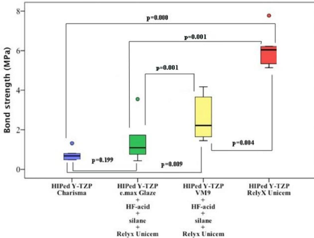
Fig. 3. Box-plot diagram comprising the bond strength (MPa) of the four studied groups. Six specimens in each group. A horizontal line within the box presents the median. Data are presented as medians, 1<sup>st</sup> and 3<sup>rd</sup> quartiles. The maximum and minimum values are illustrated via the upper and lower strokes. (•) Marks outliers.
