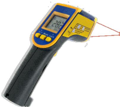
**Figure 1.** The infrared light thermometer with dual laser points.
