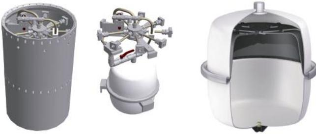
Figure 1. A 3D CAD of the NISSE experiment. Left: Mounted inside the rocket modules; Centre: Without modules; Right: 12-l Airfix A12 tank by Flamco.
