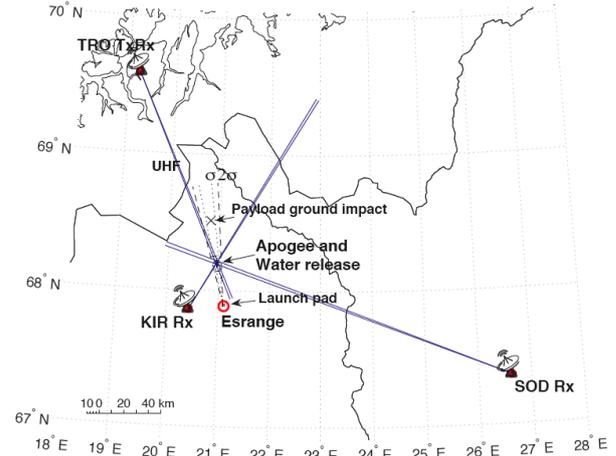
Figure 3. A schematic presentation of the REXUS 6/NISSE – EISCAT measurement configuration during the launch. The  $\sigma$ - and  $2\sigma$ -deviations from the predicted trajectory of earlier REXUS 3 are marked by dotted and dashed sectors, respectively, and are shown just for example (taken from [20]).
