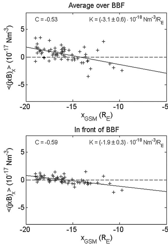
**Figure 2.** Averages of the  $x$  component of  $\mathbf{j} \times \mathbf{B}$  (in the GSM coordinate system) for the 67 events of the study, as a function of  $x_{\text{GSM}}$ . The top plot shows the average over the BBF event, the bottom plot shows the average over 15 min before the BBF event. The correlation coefficients  $C$  and the slope  $K$  of the resulting linear fit (and the standard error), which is also indicated by the solid line, are shown.
