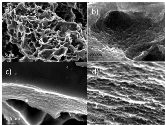
Fig. 2. SEM images recorded from a-r-GO sample with BET surface area of ~3300 m<sup>2</sup>/g. The images show hierarchical size pore network (a, b) and also some layered structure on broken grain edge (c, d).
