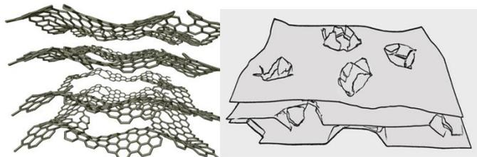
**Fig. 6.** Schematic representation of possible a-r-GO structure consisting of strongly defected fragments of graphene flakes (a) and more general scheme how the ruptured hole edges can serve as “pillars” for graphene scaffolds.
