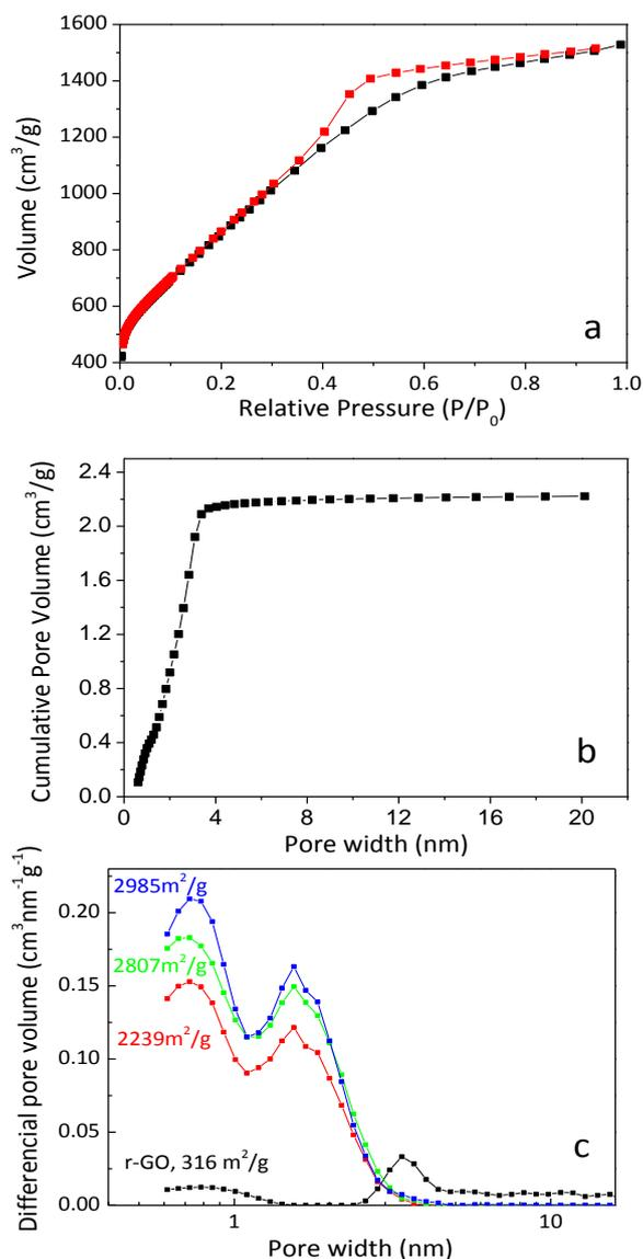
Fig. 1. N<sub>2</sub> adsorption/desorption isotherm for a-r-GO sample (SSA=3300 m<sup>2</sup>/g) (a) and analysis of isotherms simulated using QSDFT slit pore model: plot of cumulative pore volume (b), pore size distribution (c)
