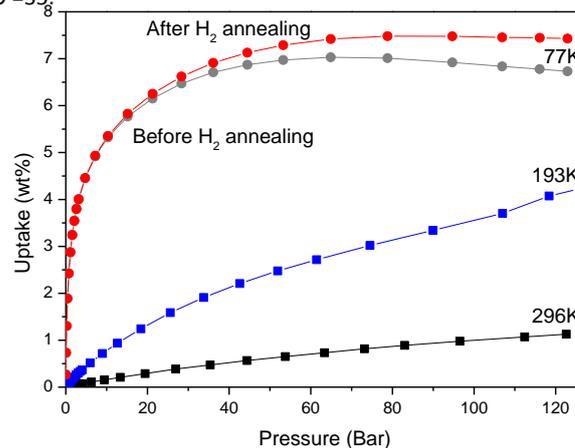
Fig. 3. Excess adsorption isotherms at T=77 K, T=193K and T=296 K for the a-r-GO sample with SSA=3230 m<sup>2</sup>/g and isotherm recorded at 77K after H<sub>2</sub> annealing.
