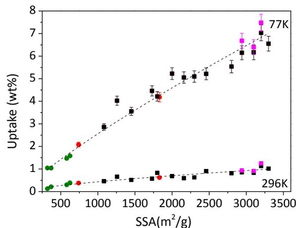
**Fig. 5.** H<sub>2</sub> uptake (wt%) vs SSA trends evaluated using volumetric method and immersion cell for a-r-GO samples at 296 K (120 bar) and 77 K (saturation value) before (■) and after H<sub>2</sub> annealing (■). The trend is extended showing samples of r-GO (●)<sup>13</sup> and reference points for Mesoporous Carbon and Activated Carbon (●).
