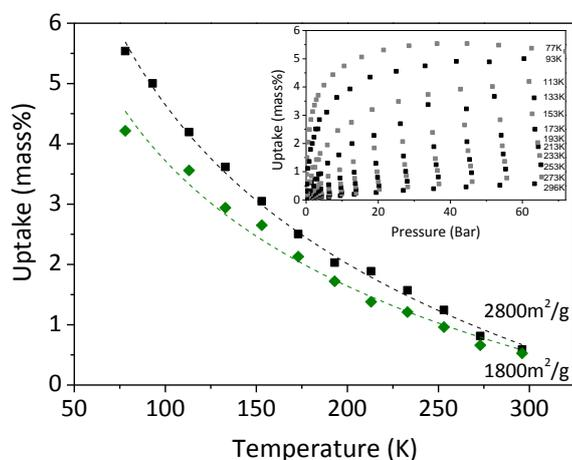
**Fig. 4.** Temperature dependence of H<sub>2</sub> uptakes for two a-r-GO samples. Inset shows isotherms recorded for a-r-GO sample with 2800 m<sup>2</sup>/g BET surface area at different temperatures up to the pressure of 65 bar H<sub>2</sub>. Isostatic heat of adsorption value of 6.1 kJ/mol was determined for this sample.
