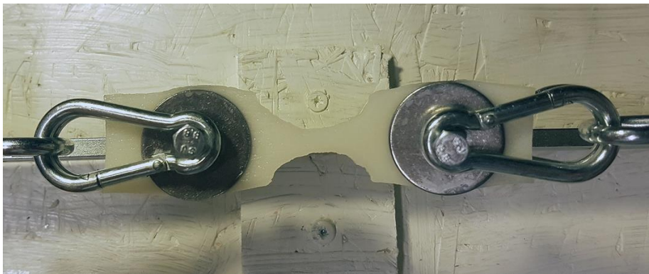
Fig 9. A Xenmatrix™ sample, cut to the dumbbell shape and mounted in the test frame.
