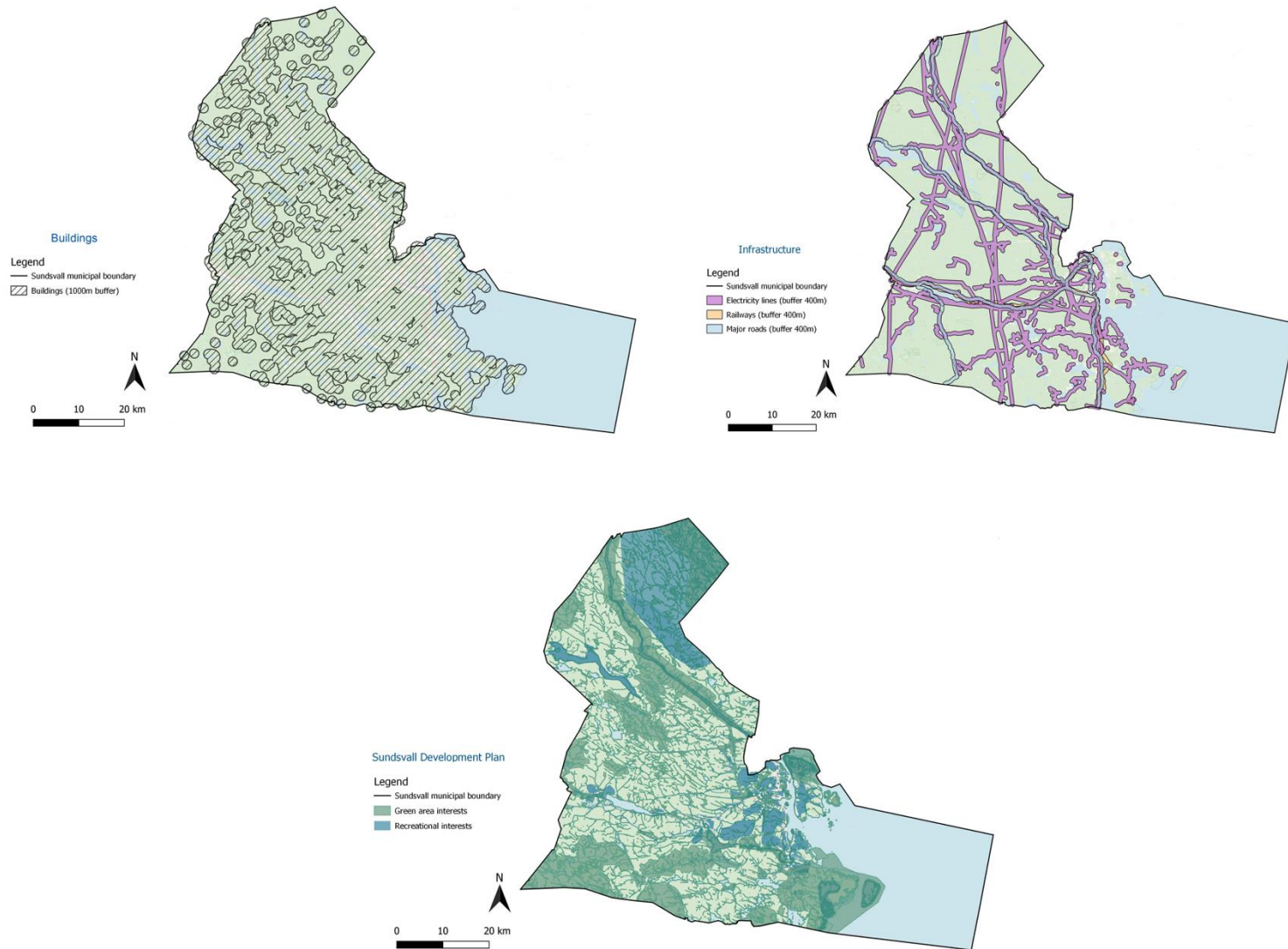
Figure 2(c): Themes 7, 8 and 9 showing the buildings (left), infrastructure (right) and Sundsvall Development Plan (middle). The constraint maps show that turbines should not be built in any coloured areas (constraint areas) based on the data in the themes.
