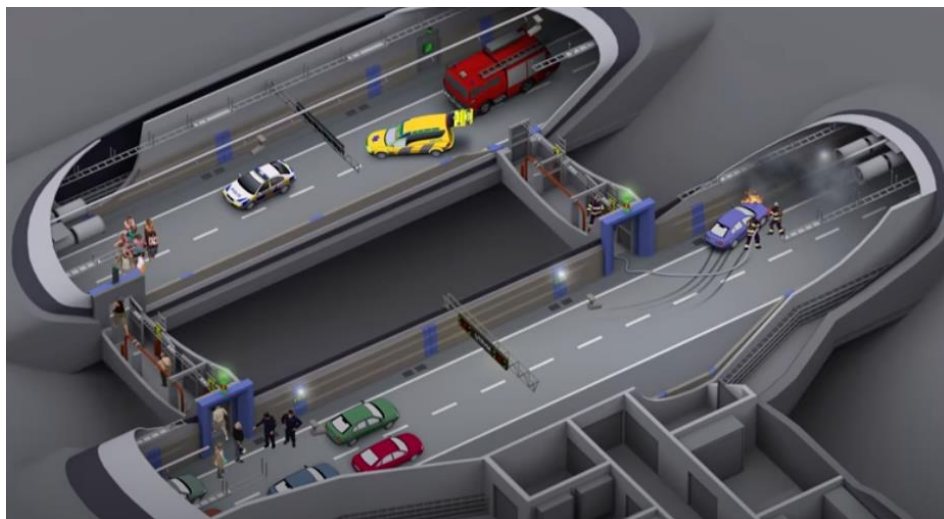
Image III. Positioning and tasks of the emergency services during a road tunnel fire. Illustration: Swedish Transport Administration (90)
