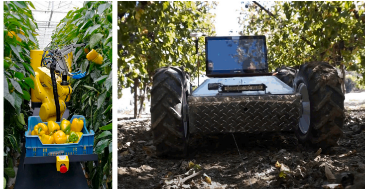
Fig. 1. Agricultural robots employing RGB-D sensors for site specific tasks. Left: SWEEPER- sweet pepper harvesting robot. Source — http://www.sweeper-robot.eu/ (Arad et al., 2020); Right: Yield estimation robot in vineyards described by Kurtser et al. (2020b).
