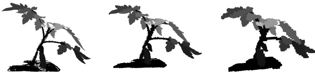
Fig. 6. Example of a point cloud acquired using a Perceptron Scan Works V5 in laboratory conditions, including discretization errors generated as a result of translation from point clouds to voxels. The point clouds are colored according to an annotation mask provided in the dataset. Left — original point clouds. Middle — discretization into voxel size = 0.01 m. Right — discretization into voxel size = 0.03 m. The images show less significant structural artifacts generated by quantization of both error points acquired compared to point clouds generated from images collected in field conditions (see Fig. 5 ). Increase in voxel size shows significant structural disruptions. Point cloud source: Schunck et al. (2021) .
