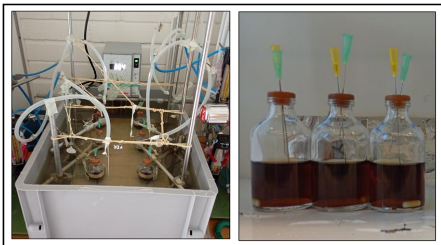
Fig. 11. A modified laboratory reactor for fermentation experiments.
