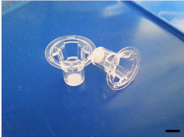
**Figure 8** The Transwell™ inserts used in studies I and II. The inserts are cell culture wells, which have a water-permeable membrane as a bottom. The membrane allows nutrient flow also for the lower part of the neotissue cultivated inside the insert. The inserts were placed in a standard 24-well plate well for the culture period. The culture medium was poured in both the well and on the top of the tissue maturing in the insert. Scale bar = 6 mm.
